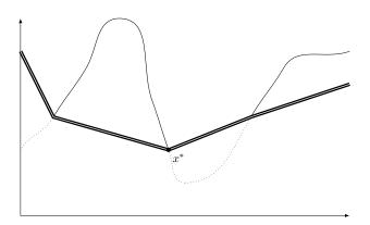
A penalty is applied. We obtain a new function that can be optimized without constraints. We find the optimal solution  $x^{\circ}$  below. We notice that this solution is not in S. This is normal; in the unconstrained problem, we can return a solution outside of S. The goal of the penalty is to be sufficiently high to avoid it.
